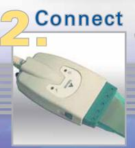
Edge Connect sensor; USB Connection to PC
